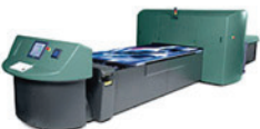
Columbia Turbo from Inca - 2 Printable area 50"W x 120"L UV based ink system Prints flexible & rigid substrates up to 1.5" thick and 1000 dpi
